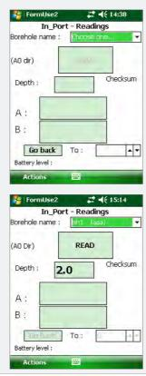
When you have chosen the borehole, tap the 'Read' button or press the Key Fob to initiate the reading process.
