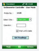
When this screen is first entered, the Field PC will interrogate the inclinometer reel and retrieve the probe calibration data from it to apply to the readings. If there is any problem with this step, the 'Get Readings' button will not be available. If the problem is with the data returned from the reel, an appropriate error message will be displayed.
