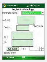
Once the borehole has been selected, the depth of the installation will be displayed along with the A and B readings. When the A0 direction has been read and the probe is rotated to read the A180 direction, the checksum box will present the opposing readings.
