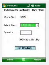
When you have selected the relevant information, click the 'Get Readings' button. If you have multiple boreholes set up within the site, use the drop-down menu to select the first borehole to be read.
