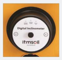
The control panel contains three coloured LED lights that display the battery, comms and power status.
