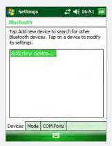
The Field PC will search for available Bluetooth devices and provide you with the accessible choices. There may only be one device shown; the Digital Inclinometer System itself.
